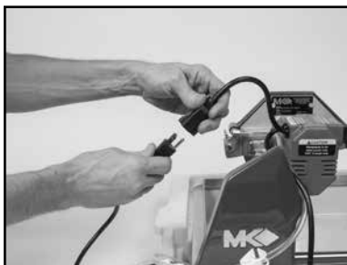
(E) Connect the Water Pump power cord to the connection found on the back of the motor.
