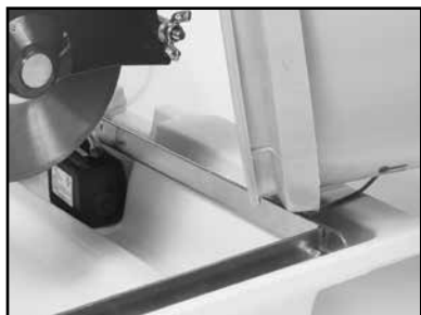
(D) Fill the Water Pan with clean water covering Pump suction (this should be done periodically during cutting).
