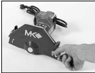
(B) Remove the Blade Guard Wingnut and then remove the Blade Guard.
