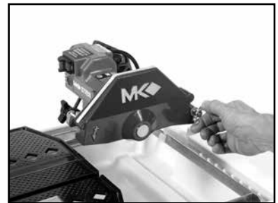
(F) Install the Blade Guard and tighten Wingnut and Retaining Knob.
