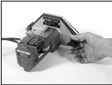
(A) Loosen the Blade Guard Retaining Knob.
