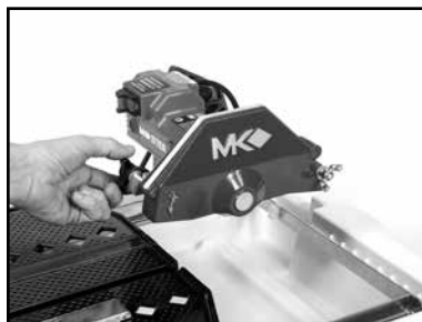
(B) Loosen the Blade Guard Retaining Knob and open the Blade Guard.
