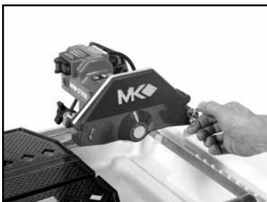
(A) Loosen the Blade Guard Retaining Wingnut.
