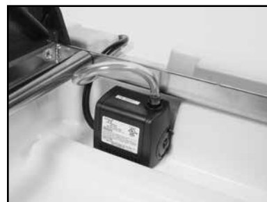
(C) Place the Water Pump in the Water Pan with the suction down and insert the Pump Cord to the clip in the back. Ensure pump is against back of water pan.
