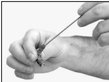
(E) Clean the Blade Guard Intake Fitting.
