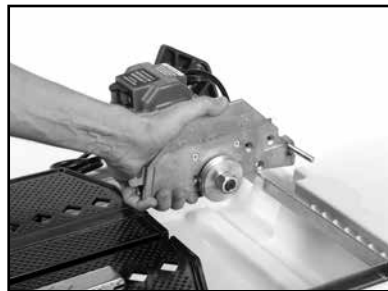
(D) Align the Cutting Head Retaining Holes to the holes on the Post.
