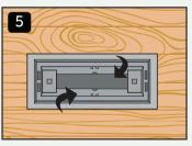
To adjust airflow, remove **tray** and bend dampers. For optimal air flow, push dampers past 90°.
