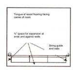
Leave a ¾" expansion gap at each end. Set nails and fill holes with matching putty. Pome
