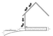
NOTE: Proper drainage away from the structure is absolutely critical to ensure weather-tight conditions and crucial to proper hardwood flooring performance. If structure is near a hill, the lot should be graded with a swale to move moisture off the lot and prevent it from coming in contact with the foundation.
