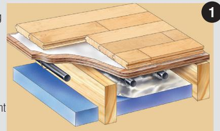
The **second method** is used when hardwood flooring boards are to be installed on an already existing floor, or when it is impossible to install the radiant heating system between the floor joists. This method consists of installing the hardwood flooring boards on a new sub-floor covered with vapour barrier paper and supported by the ledger strips of the old flooring. The radiant heating system is installed between the ledger strips.
