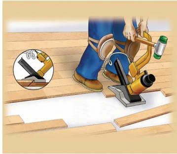
Both the conventional floor nailer and finishing air-hammers must be calibrated according to manufacturer's specifications. To verify compliance with manufacturer's specifications, test the tools on a piece of scrap wood in order to avoid damaging good boards. This method will avoid damage to boards resulting from too much air pressure, too much physical pressure applied to boards or misuse of the air-hammer.
