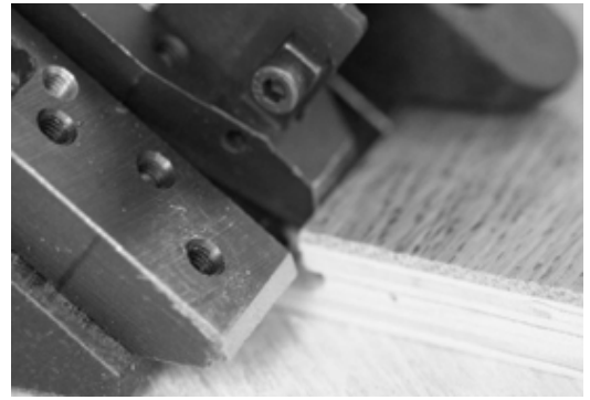
Fig. 13 Pushed in to the groove = correct position
