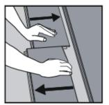
Separate the whole row by lifting it up delicately at an angle. To separate the planks, tilt slightly and slide them apart.
