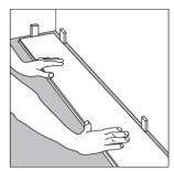
1. After thoroughly cleaning the subfloor, you should begin laying in the left-hand corner. Place the floorboard 10mm (1/2") from the left wall. Use spacers between the Wall and the floorboard.
