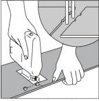
9. **Holes for pipes:** measure the diameter of the pipe and drill a hole that is 20mm (7/8") larger. Saw off a piece as shown in the figure and lay the board in place on the floor Then lay the sawed-off piece in place.
