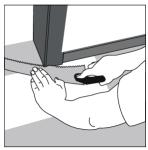
10. **Door molding and skirting:** lay a board (with the decorative side down) next to the door molding and as shown in the figure, and cut using a hand saw or equivalent. When installing, slide the plank under themolding.
