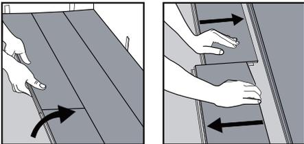
Separate the whole row by lifting it up delicately at an angle. To separate individual plank end-joints within a row, leave them flat on the ground and slide them apart. If planks do not separate easily, you can slightly lift up the planks (5° angle) when sliding them apart.
