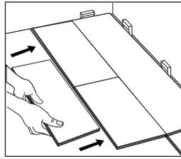
When installing each new row, take a full loose plank and use the long side to tap against the prior row to ensure there is no gapping.
