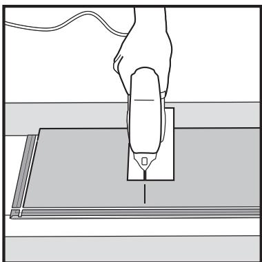
**4** If cutting with a jig saw, the laminate surface should be turned down. If cutting with a hand saw, the laminate surface should be face up.
