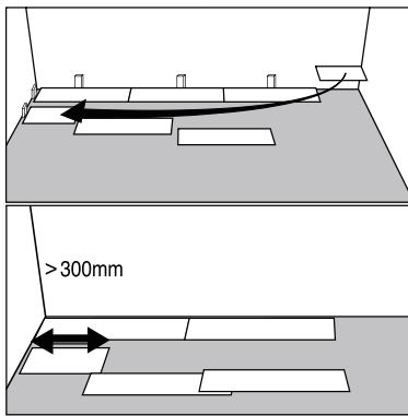
**5** Start the second row with the leftover cut part of the last plank of the previous row. This small plank should measure at least 12" (30cm). Otherwise, use another plank that should be cut in two. Short pieces should be cut to at least 12" (30cm).
