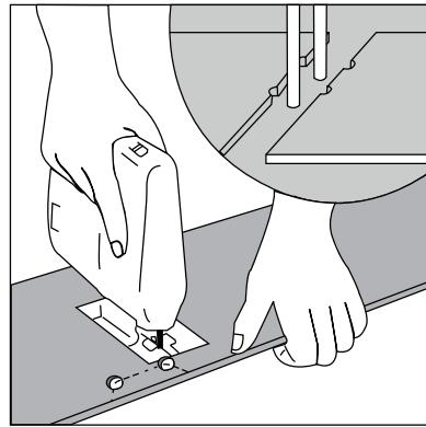
**9** Holes for pipes: measure the diameter of the pipe and drill a hole that is 7/8" (20mm) larger into the plank. Saw the plank into two pieces perpendicular to the length and bisecting the previously drilled hole. Then lay the two pieces in place around the pipe.
