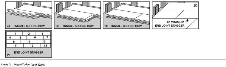
• Use the pull bar to draw the last row to fit tightly to the previous row.
