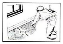
Use Tapping Block if necessary to fit planks snug together at side and butt ends. Clean any adhesive off the surface before it cures using clean terry cloth towels and mineral spirits.
