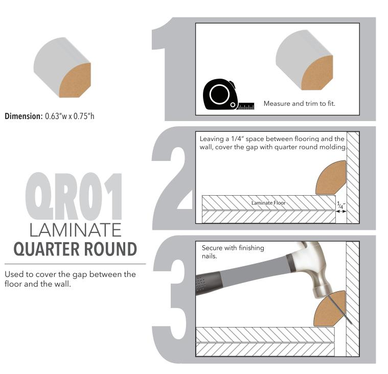
Surface: Wear resistant laminate Core Material: Moisture resistant MDF
