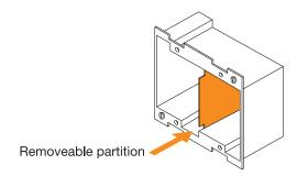
Install gang boxes that include vertical partitions (available at local electrical distributor) unless Class 2 circuit conductors are installed (NEC: in accordance with 725.41 Class 1 Circuits).
