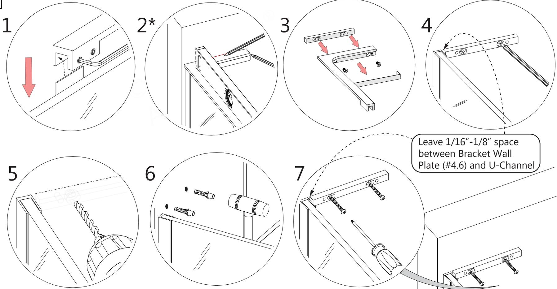
Leave 1/16" - 1/8" space between Bracket Wall Plate (#4.6) and U-Channel
