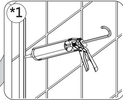
\*Fast-drying 100% silicone recommended for the installation of hinge panels.
