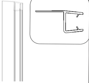
Vinyl Seal with Flexible Fin for 10 mm (3/8") glass **x1**
