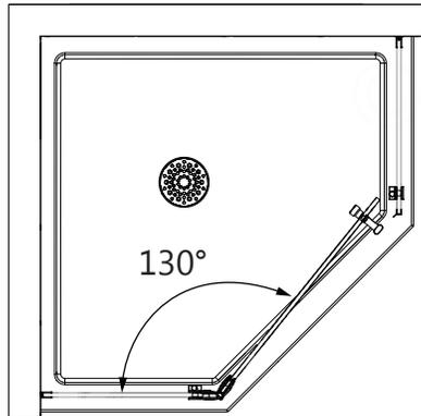
The Adjustable Hinge Assemblies are factory pre-set to overclose to 130° to create a tight seal with the Strike Vinyl. If strike vinyl is not used, the hinges can be adjusted to close to a different angle (135° for example).
