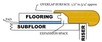
Overlap Stairnosings/moldings are milled to allow the "lip" to ride up over the top of the flooring; used primarily with floating floor applications.
