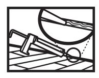
After installing planks and before installing trim, remove all spacers. Create a water tight spacing applying 3/8" PE foam backer rod and 100% flexible silicone sealant along the entire perimeter of room and around fixed objects and transitional moldings. Do not use acrylic sealant.
