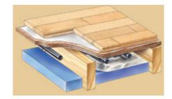
The **second method** is used when hardwood flooring boards are to be installed on an already existing floor, or when it is impossible to install the radiant heating system between the floor joists. This method consists of installing the hardwood flooring boards on a new sub-floor covered with vapour barrier paper and supported by the ledger strips of the old flooring. The radiant heating system is installed between the ledger strips.
