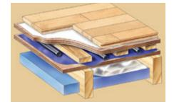
The **fourth method** involves installing the hardwood flooring boards on a radiant heating system installed directly in a concrete slab, either in a sub-floor or a building with concrete floors. A sub-floor consisting of two 1/2 in (1.3 cm) sheets of interlocking plywood covered with vapour barrier paper is then installed directly on the concrete. This type of installation is often referred to as a floating floor.
