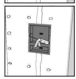
6. Neatly apply 100% waterproofing silicone to cover each screw head and to fill the gap between the niche flange and the adjacent shower board.
