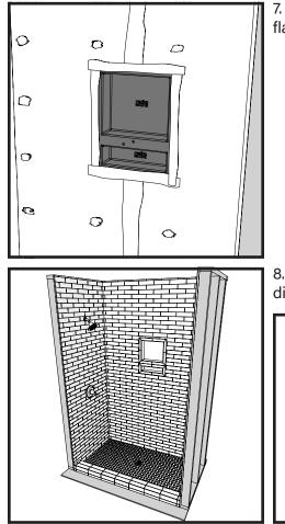
7. Then apply a liquid applied waterproofing membrane to all four niche flanges and covering at least 1 inch of the adjacent tile backer board
