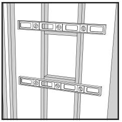
3. Measure and cut top and bottom horizontal support framing to a length which permits each to run between and to be fastened to both vertical studs. Level and mechanically fasten the top and bottom horizontal support brackets to both adjacent vertical studs so that the vertical dimension between the horizontal support framing matches the vertical dimension of the pre-drilled fastening holes on the Redi Niche flange.
