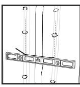
a. Place the niche between the two marked studs with the flange walls flush against the wall and trace the outline of the niche on the wall. Be sure the top and bottom lines are level.
